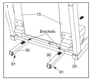
With the help of a second person, carefully tip the Uprights (20) and the Walking Platform (not shown) down to the position shown. Make sure that the Extension Legs (90) remain in place.
